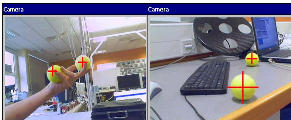
**Fig. 3 Colour ball detection using optical sensing**
