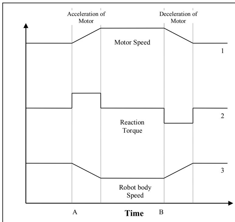
**Fig 2: Graphs showing speed of motor, robot body and reaction torque on robot body during the process of finding coloured pixel and keeping it in the middle of screen**
