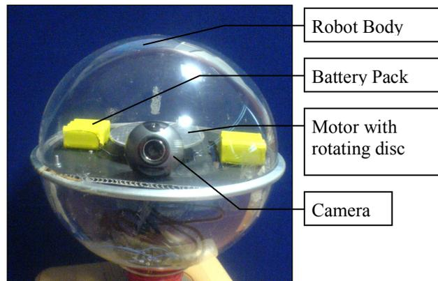
**Fig. 1 Robot body showing layout of the components mounted in it**
