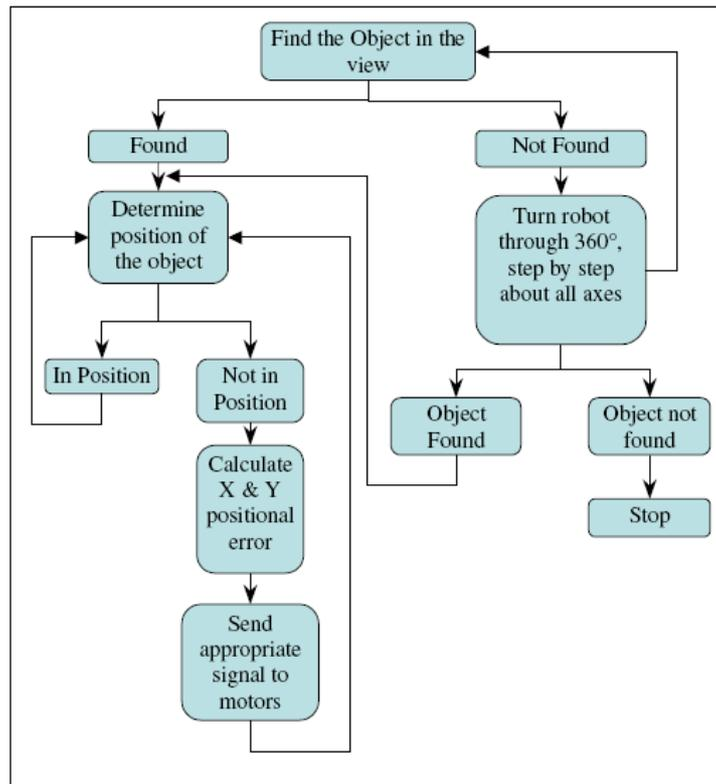
**Fig. 4 Flowchart for program of robot**
