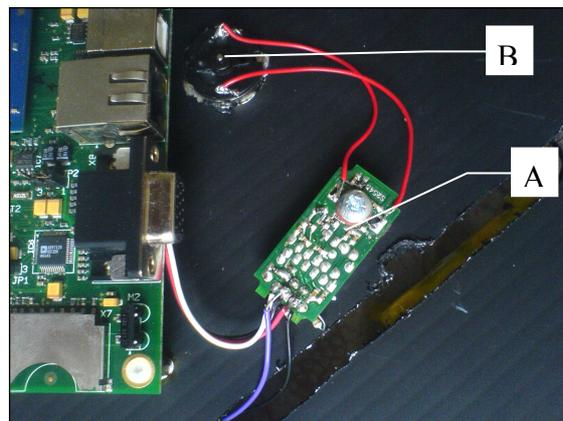
**Fig. 5 Modified servo motor card and normal DC motor attached to it, whole assembly mounted on the robot**
