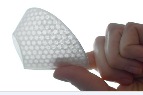
This ongoing research is based on developing a new way of producing lampshades by 3D printing recyclable PLA straight onto fabric in order to reduce plastic waste.
